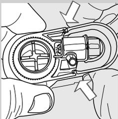
**22** Attach the Automatic Milk Frother to the fitting and ensure it is locked into place in the seat.
