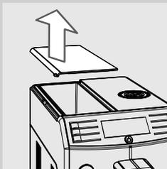
**4** Lift the water tank using the handle.
