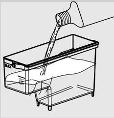
6 Remove the water tank and pour the entire content of the Descaling solution. Then fill the water tank with fresh water up to the calc clean level.
