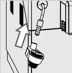
**25** Insert the Automatic Milk Frother until it locks in place on the rubber grip.
