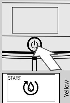
**13** To turn on the machine simply press the "⏻" button. The control panel indicates that the circuit must be primed.
