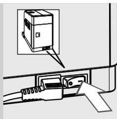
**12** Switch the power button to "I" turn on the machine. The "⏻" button blinks.
