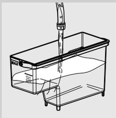
12 Remove the water tank, rinse it and fill it up to the MAX level with fresh water. Place it back into the machine. When inserting the water tank into the machine, the display below is displayed.
