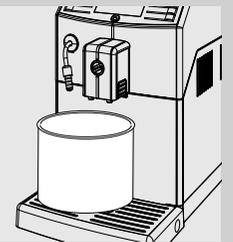
8 Place a large container (1.5L) under both the steam/hot water wand and the dispensing spout.
