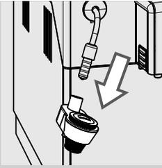
2 Remove the Automatic Milk Frother from the hot water/steam wand.
