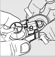
**18** To detach the Automatic Milk Frother, press the sides and remove it by applying light lateral movements as shown in the figure.
