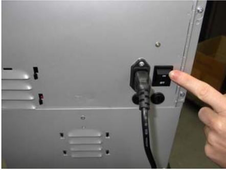
A starting switch placed in the rear part of the machine cuts the power off all electrical and electronic components in the machine.
