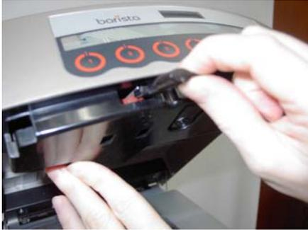
A safety switch is provided in the machine, **which cuts the power off to all 24 V supplied components in the machine when the door is opened.** Then **insert the safety key** into the safety switch as shown in the picture.
