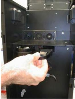
and the aspiration drawers. Immerse all parts in the solution. Using a cloth soaked in the solution, proceed to clean also the attachment bases of the mixers, which remain fixed to the machine. The time of permanence in the solution, in order to obtain a full disinfecting, is stated on the packaging of the chemical
