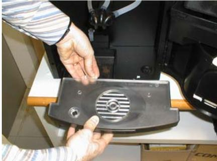
Remove the liquid waste bucket,
