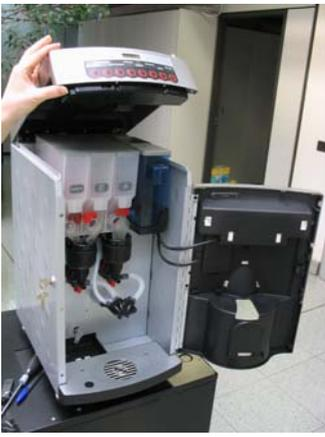
Open the front door and lift the cover. completely the canisters
