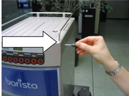
The machine is controlled by a program stored in the microprocessor of the FLASH memory, installed on the CPU board. The program stored in the memory (**master file**) can be updated with **Rhea black flash card** programmed with the Rreaction Program.
