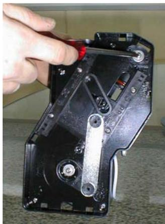
Remove the plates of the superior filter
