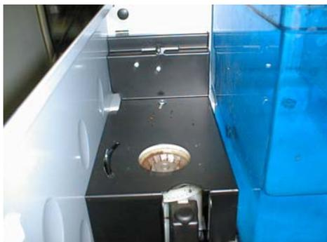
The brewing time for a 50 ml espresso coffee must be around 20 sec. If due to the wear and tear of the grinder, the brewing time is shorter, turn the adjustment ring nut of the grinder by 1-3 steps in the direction indicated by the sticker near the grinder itself. A thinner grinding and therefore, an adequate brewing time id then obtained.
